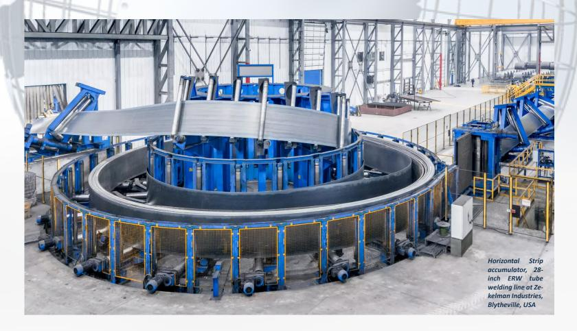
ekelman Industries and SMS group write history with the world's largest continuous 28-inch ERW tube welding line with wall thicknesses of up to 25.4 millimeters.
